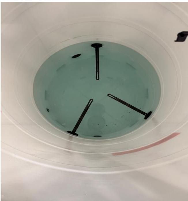
View of Heating Elements from the top of the CIP Tank:
